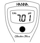
When "7.01" blinks on the display, place the tip of the probe into a pH 4, 7, or 10 buffer solution.
