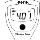
If pH 4 or 10 buffer solution is used as the first point the value of the buffer is recognized and displayed with the blinking stability indicator.
