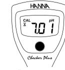
If pH 7 buffer solution is used as the first point the buffer is recognized with the blinking stability indicator.
