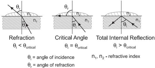
In the HI 96811, light from an LED passes through a prism in contact with the sample. An image sensor determines the critical angle at which the light is no longer refracted through the sample.
