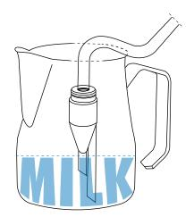
Fill the jug to the point where the milk just touches the central tube of the silicone
