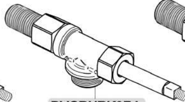
DVGRUBK3F-L Asta filettata e prolunga / Threaded rod and extension
